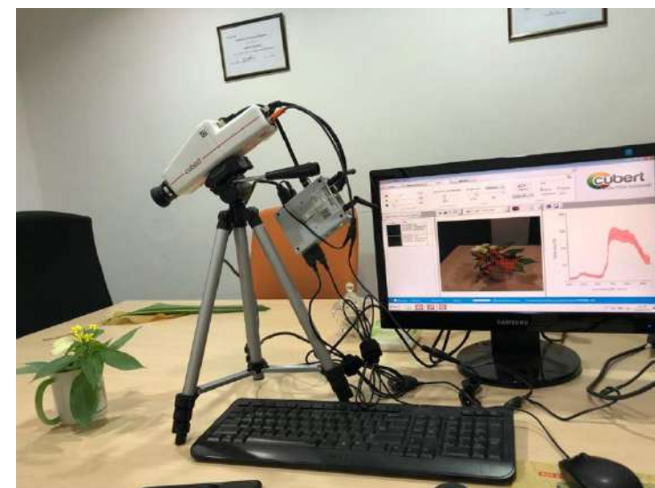
Spectral measurement on leaves (yellow box)
