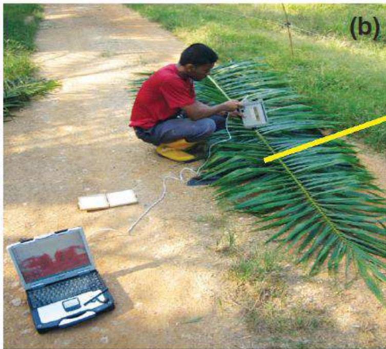
Spectral measurement on leaves (yellow box)
