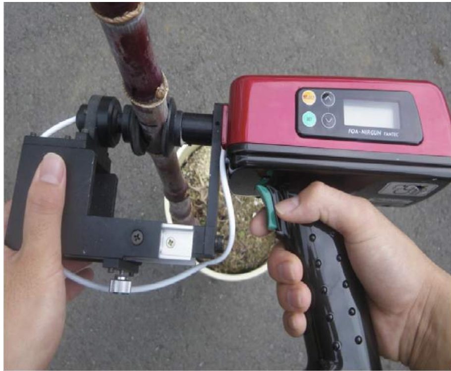
Figure 1. Non-destructive cane measurement using a portable NIR (near infrared) spectrophotometer in transmittance mode.
