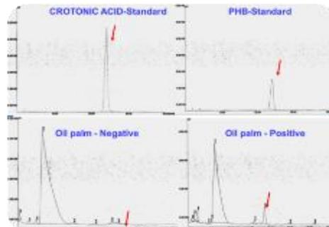
Detection of PHB in the form of crotonic acid by HPLC.
