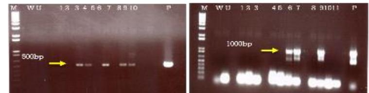
PCR analysis using Hygrec primers (~500bp). Five out of ten samples obtained band, from sample number 2, 4, 6, 8 and 9.
