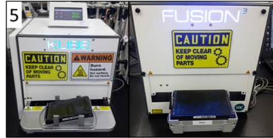
5 Plate sealing ❖ Thermal and laser sealing of plates
