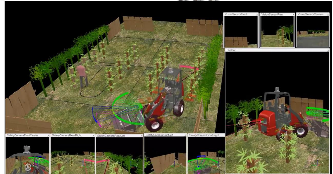
Human collision avoidance with Long-range and short-range distance sensors. (c)SunBot.de, Redmond R. Shamshiri
