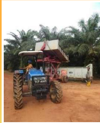
Compact Tr. - unload FFB into 10t bin
