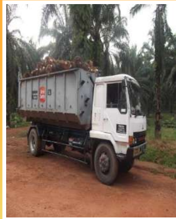
FFB lorry - cw hooklift will load the 10t bin from bin station
