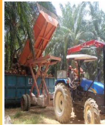
Unloading FFB into 10t bin
