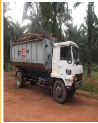
FFB lorry – cw hooklift will load the 10t bin from bin station
