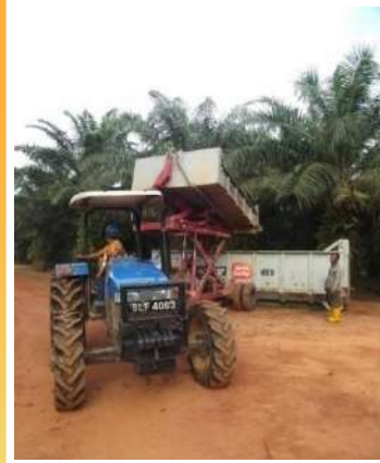
Compact Tr. – unload FFB into 10t bin
