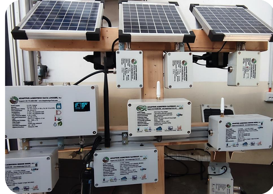
Multi-sensor platform with redundant storage
