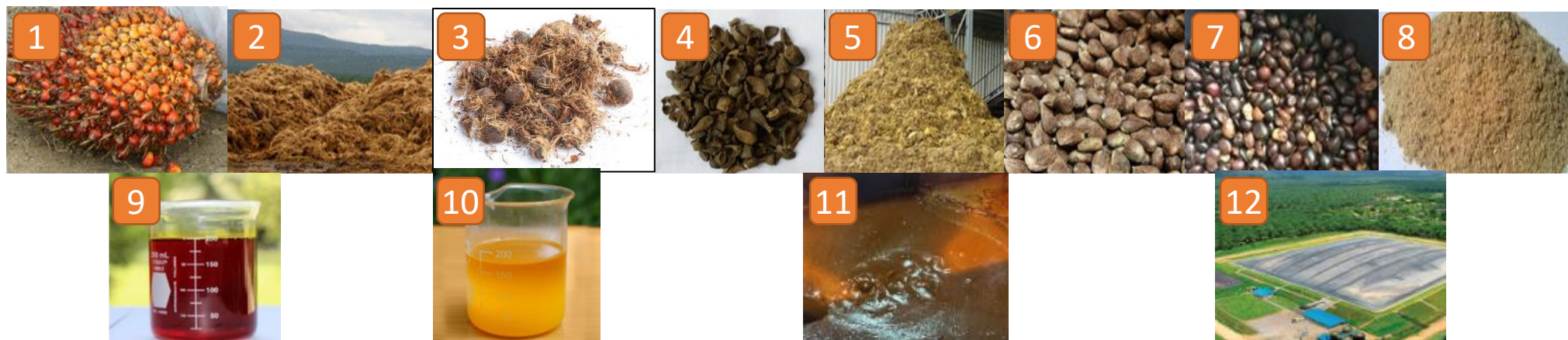
Figure 1. Main products and by-products obtained during FFB processing at palm oil mills (POMs). (1) FFB before processing, (2) EFB pressed, (3) fruit pressed with nuts and fiber, (4) cracked nuts, (5) fiber, (6) nuts, (7) palm kernel, (8) palm kernel pressed cake, (9) CPO, (10) CPKO, (11) sludge, (12) effluent treatment systems (POME).
